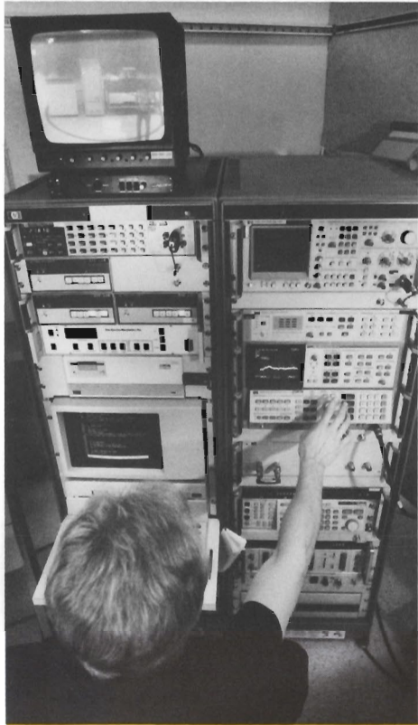
Richard Barbin can watch products undergoing EMI testing on a closed-circuit television monitor (upper left).
