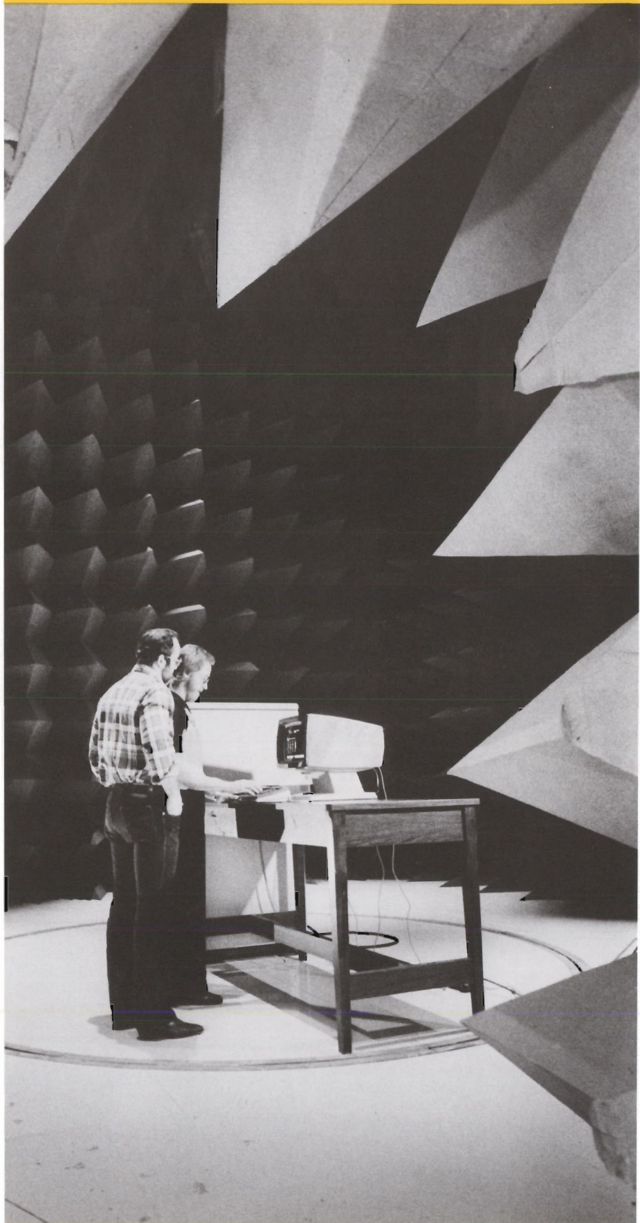
Jim Murray and Richard Barbin program an HP computer on the anechoic chamber's turntable. The turntable will spin slowly during the computer-controlled test.
